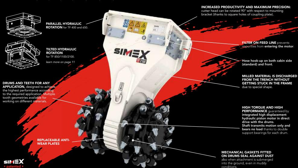
The Simex TF double drum cutter heads are ideal for trenching, profiling rock and cement walls, tunnelling, quarrying, demolition, dredging, finishing operations and underwater works. They are highly effective where conventional excavation systems are too weak and percussion ones have little effect.
